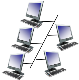
shared wire (e.g., cabled Ethernet)
