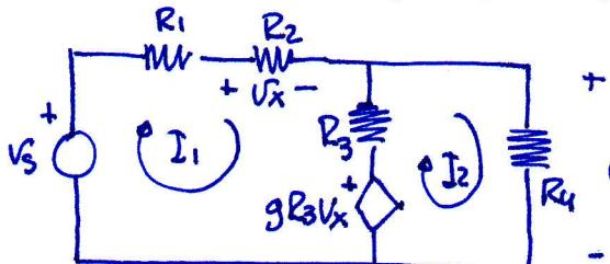
$$\begin{aligned} & \text{Plantejem 2 equacions:} \\ & V_o (R_1 + R_2 + R_3) I_1 - R_3 I_2 = V_s - g R_3 V_x \\ & -R_3 I_1 + (R_3 + R_4) I_2 = g R_3 V_x \end{aligned}$$
