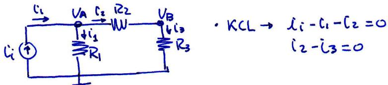
$$\begin{aligned} \text{KCL} \rightarrow i_i - i_1 - i_2 &= 0 \\ i_2 - i_3 &= 0 \end{aligned}$$
