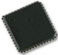
Figure 2. The Analog Devices AD9250 ADC has all the attributes required for precision conversion.
