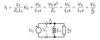
First term L<sub>1</sub> depends on the magnetic coupling. No dc!
