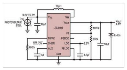
Figure 2: Single photovoltaic cell Li-Ion trickle charger
