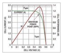
Figure 4: Typical maximum power point control point for a single photovoltaic cell
