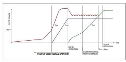
Figure 3: Typical LTC3105 start-up sequence
