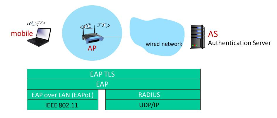
Extensible Authentication Protocol (EAP) [RFC 3748] defines end-to-end request/response protocol between mobile device, AS
