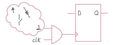
2. (3 points) We want the input number 1 of the IC 74HCT00 to be at logic zero, except when a *normally* open switch is pushed (i.e. short-circuited). Use a *pull-up* or *pull-down* resistor based design to achieve this behavior completing the following circuit.
