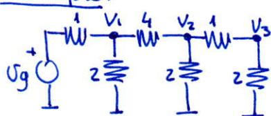
$$\frac{v_1 - v_g}{1} + \frac{v_1}{2} + \frac{v_1 - v_2}{4} = 0$$
