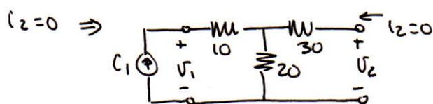
$$V_1 = 10i_1 + 20i_1 = 30i_1 \Rightarrow R_{11} = \frac{V_1}{i_1} \Big|_{i_2=0} = 30$$
