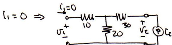
$$V_1 = 20i_2 \Rightarrow R_{12} = \frac{V_1}{i_2} \Big|_{i_1=0} = 20$$
